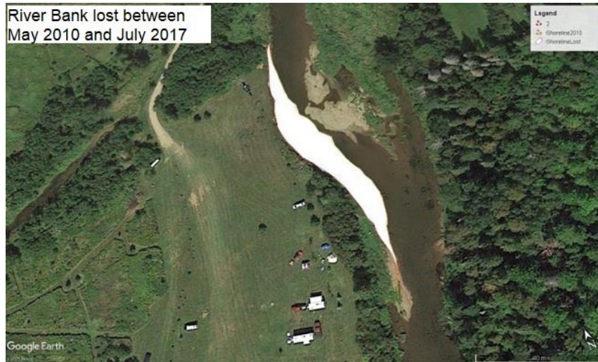
Figure 20: Area of bank lost at this site between 2010 and 2017: 1,235 m 2
