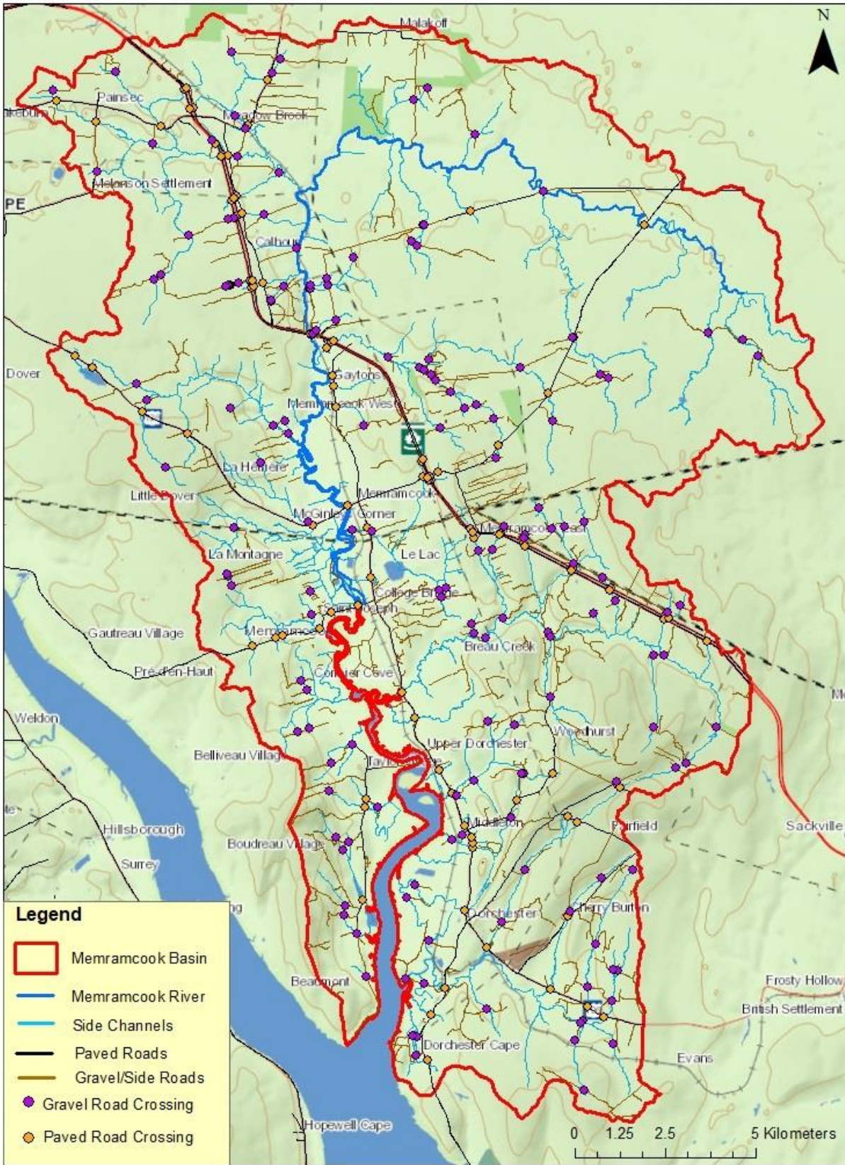
Figure 2-6: Road network and water-crossings within the Memramcook Watershed.
