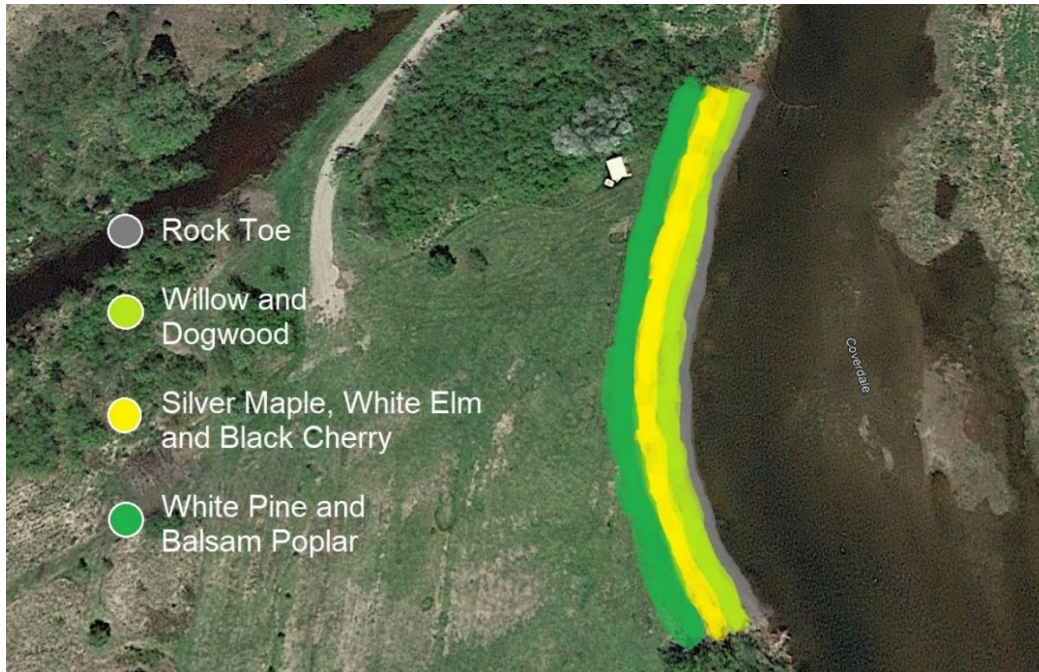
Figure 23: Distribution of vegetation planted at 2017 site
