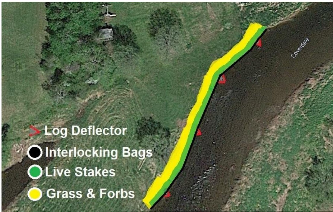
Figure 27: Distribution of vegetation planted at 2022 site
